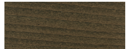
Art.-Nr.: JC7320-8153 (Green Mate) 93 T farblos, 2 T gelb (p), 2 T rot (p), 1 T blau (p), 2 T schwarz (p)
